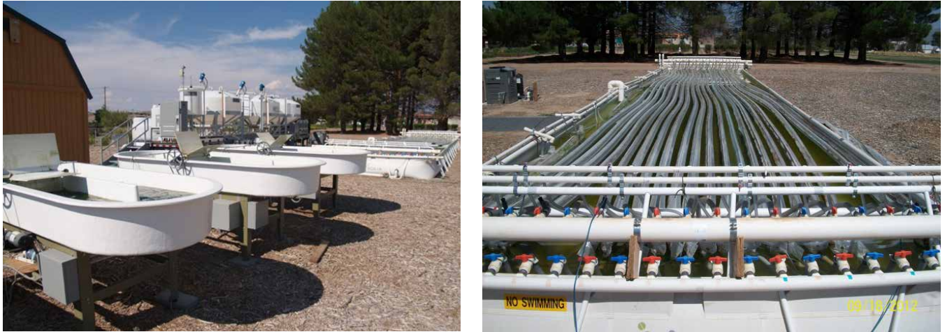
Figure 3. NMSU Testbed Culture Systems: (a) traditional paddlewheel systems and (b) Solix PBR system
