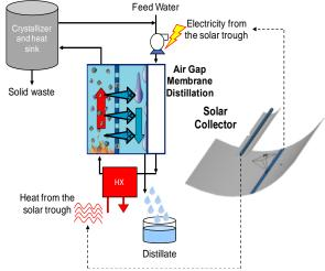
Figure 1. Hybrid CSP/PV solar collector coupled with MD. The hybrid solar collector generates heat and electricity for the air-gap MD system.
